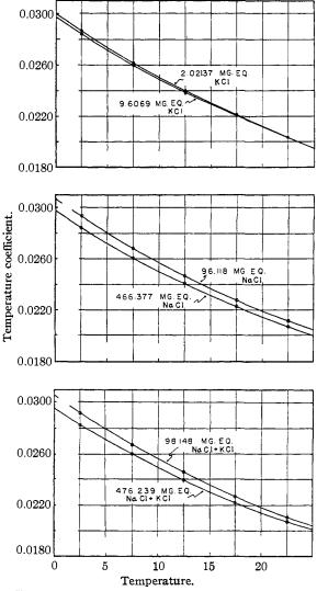
Fig. 2.—Temperature coefficients of the equivalent conductance for sodium chloride, potassium chloride and a mixture of sodium chloride and potassium chloride.
