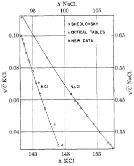
Fig. 1.—Equivalent conductance of sodium chloride and of potassium chloride solutions.
