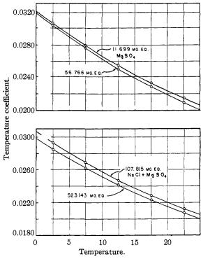
Fig. 3.—Temperature coefficients of the equivalent conductance of magnesium sulfate and a mixture of magnesium sulfate and sodium chloride.
